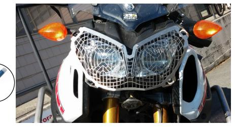
(4) Install headlight guard. **!TIP** A dab of water on each ball stud will help it fit in place easier with less wear and tear on the rubber grommets.
