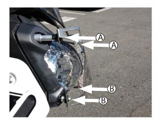
Apply a small drop of loctite to the threads of each ball stud. Thread in each ball stud to the four locations. Longer 40mm ball studs into two upper positions (A). Shorter 25mm ball studs into lower positions (B) Tighten to 6.5Nm.
