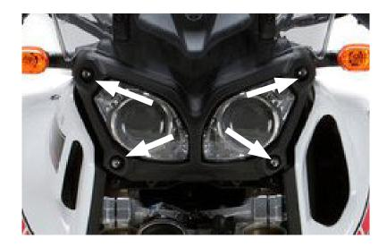
(2) Use 5mm allen and remove four screws shown.
