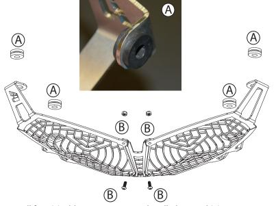
Install four (4)rubber grommets into headlight guard.(A) Use care to not rip the rubber. **!TIP** a dab of water will help them slide into place. Install M3 torx screws with lock nut (B) use T10 torx and 5.5 nut driver.
